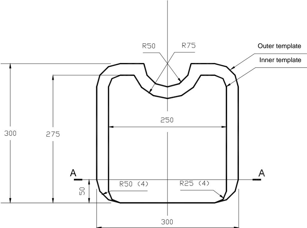
Drawing 3: Cockpit cross section template
